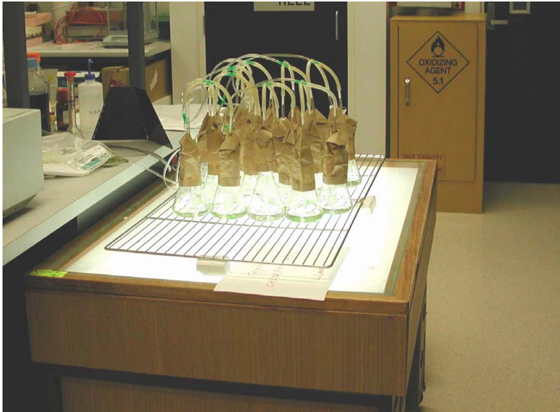
Figure 4.1.4 Setup for culturing algae on a light table.
